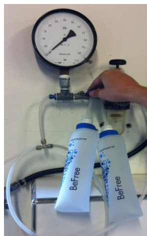
Picture 2: Burst test of softflask with pressurized air to eliminate potential leakage.
