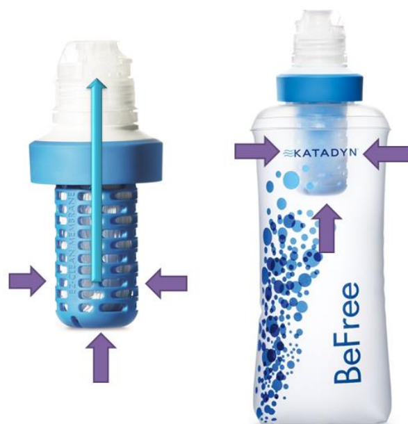
Picture 10: Open filter housing for free water access to the hollow fiber filtration unit. When the softflask of the BeFree system is squeezed, pressure pushes the water directly against the fiber membranes and clean drinking water penetrates through the membrane.
