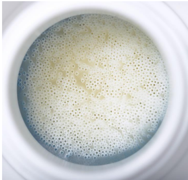
Picture 9: Open fiber ends of the BeFree system as seen from the top. Space in between the open fiber ends is blocked off and watertight.
