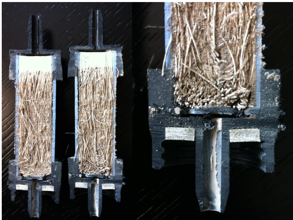
Picture 11: Hollow fiber filter with enclosed housing - inside view after 100L filtration performance: plain white hollow fibers have turned into a brown dirt trap (competitor product).
