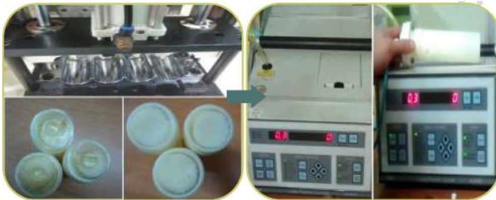
Picture 1: Particle challenge test of hollow fiber bundles with laser counter for accurate results.
