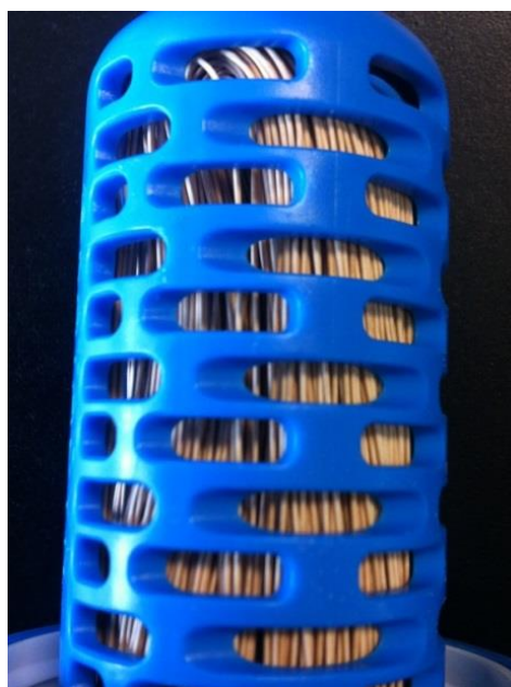
Picture 12: Close-up of the BeFree element after 1000L of filtration. Note the slight brown discoloration of the white hollow fibers. Otherwise no dirt or particles are noticeable.
